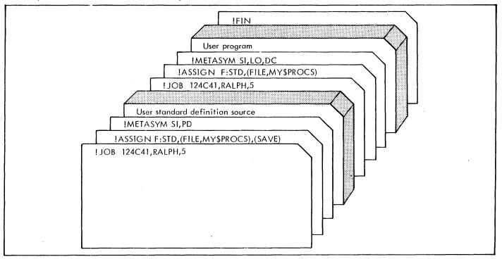
Figure 12. Creation and Use of a Named Standard Definition File
