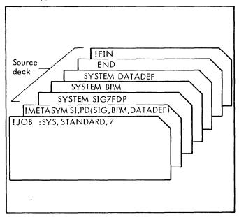
Figure 11. Creation of a Standard Definition File
