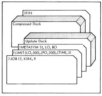
Figure 14. Sample Run Deck – Single Assembly with Update
