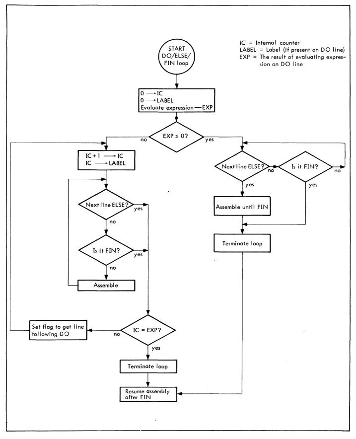
Figure 3. Flowchart of DO/ELSE/FIN Loop
