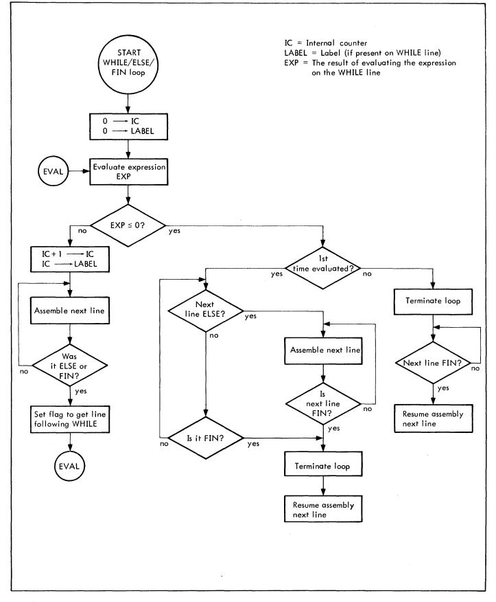
Figure 2. Flowchart of WHILE/ELSE/FIN Loop
