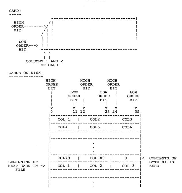
Figure B-1. Layout of Card Data That is Transferred to Disk Using the /IMAGE Switch with \$CREATE or \$DATA
