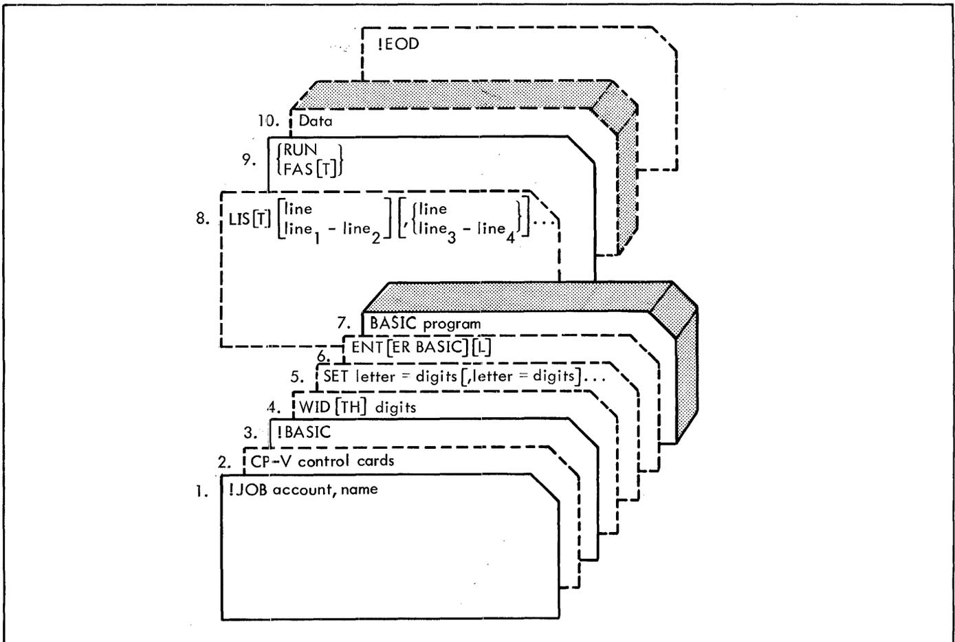
Figure 6. Deck Setup for BASIC Batch Processing (CP-V)
